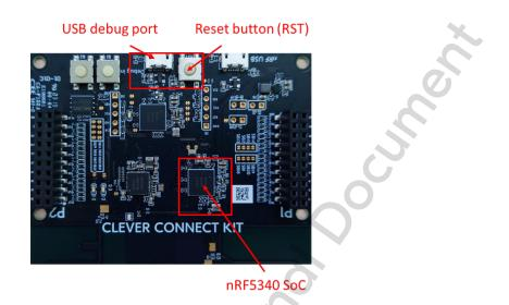
The Reset button (RST) on the board resets the nRF5340 SoC.
