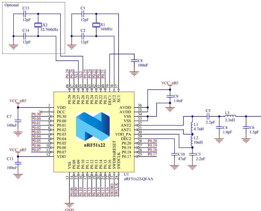
**Figure 22** QFAA QFN48 with internal LDO setup
