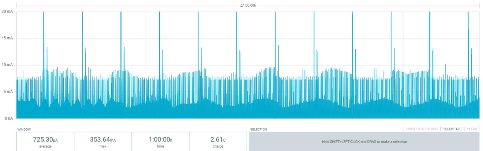
3) Here we've zoomed-in on a 3-second section of the above image showing the current draw due to BLE in the first six-hours after connecting the device to the iPhone over BLE. This is a section without any of our threads running, so the nRF52840 is in Sleep mode. Our hardware is responsible for about 70 uA of this, so roughly 180 uA are due to BLE being connected in this mode. Looks good.
