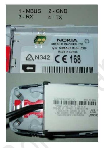
The very popular Nokia 3310/3315 has the F/M Bus connection under the battery holder. This is a bit of a pain to get to and requires a special cable to make the connection. The left picture above shows the 4 gold pads used for the F and M Bus. The right picture shows the F-Bus cable connected to my Nokia 3310.
