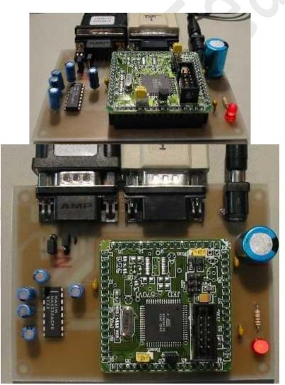
The two jumpers near the F-Bus connection sets the levels for RTS and DTR. The 6 Pin header on the AVR570 is the In-Circuit Programming (ISP) port with the 10 Pin IDC used for JTAG programming and debugging. The board was designed with hole-through components as I am trying to get rid of my old stock!
