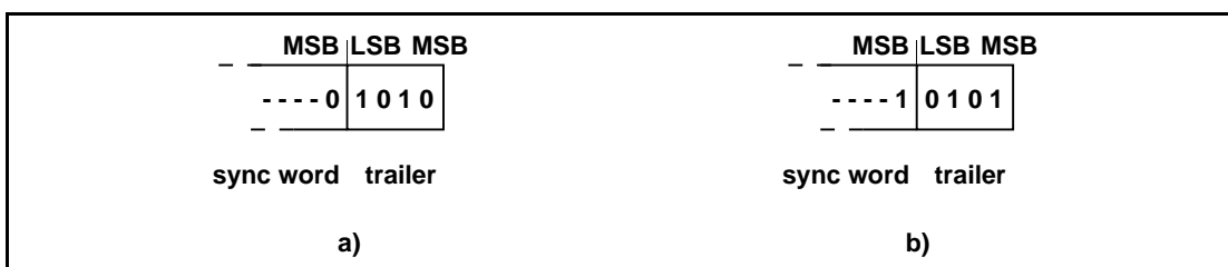
Figure 6.7: Trailer in CAC when MSB of sync word is 0 (a), and when MSB of sync word is 1 (b)
