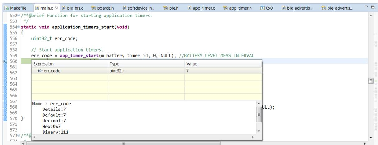
Figure 15: `NRF_ERROR_INVALID_PARAM` error. Error codes are listed in `nrf_error.h` header.
