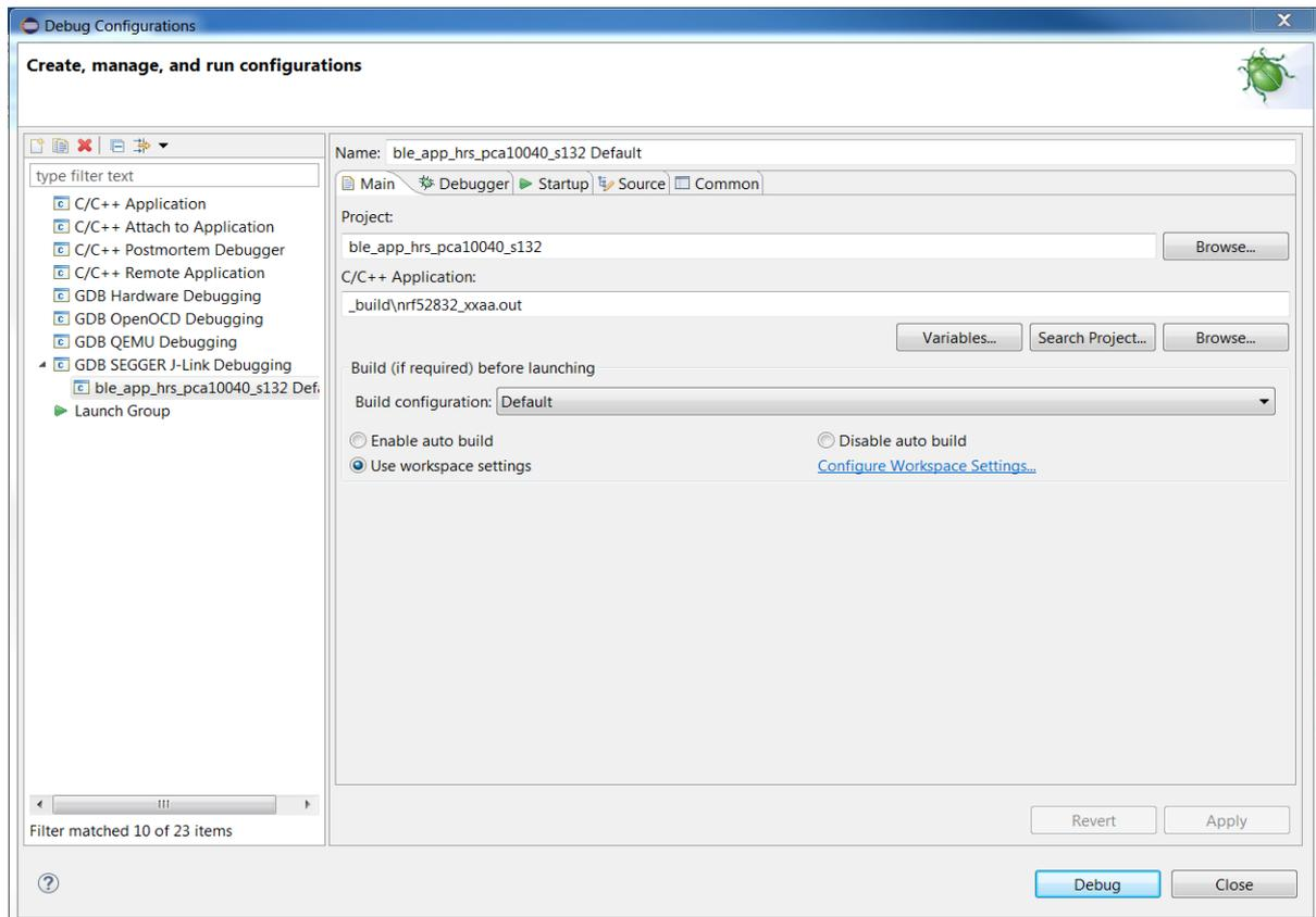
Figure 12: Main tab - check that \*.out file is set in C/C++ Application field
