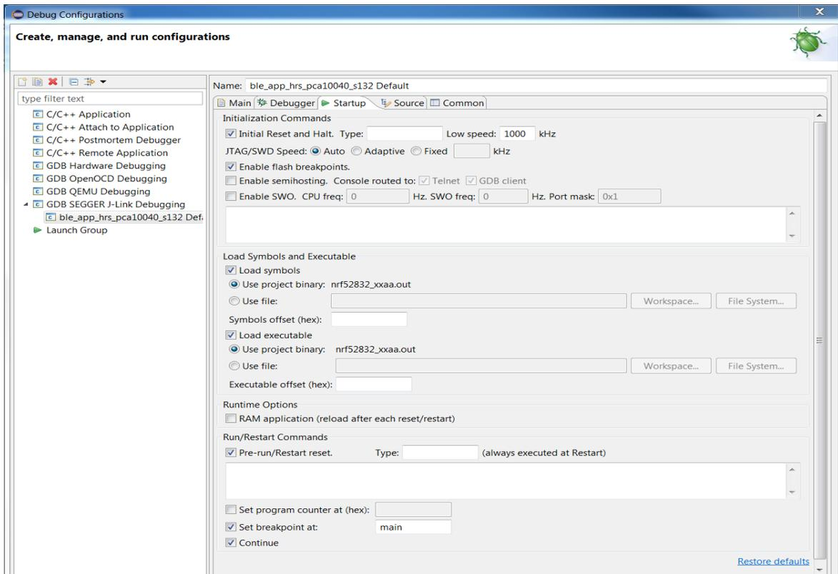
Figure 14: Startup configuration - semihosting and SWO are enabled by default, but not implemented in code examples.
