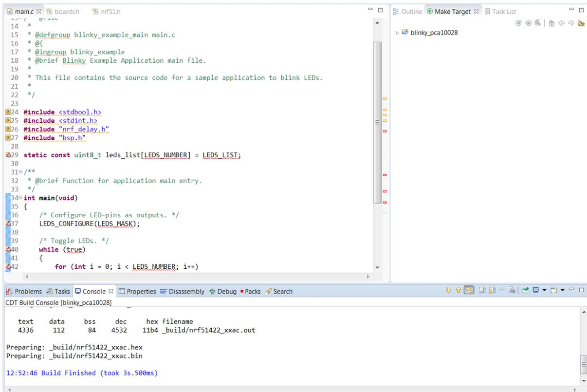
Figure 2: Successful build without errors.
