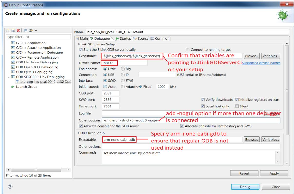
Figure 13: Debugger configuration
