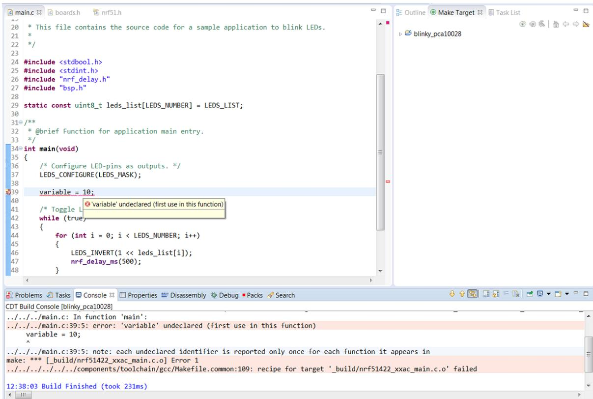
Figure 1: Build error: referencing an undeclared variable.
