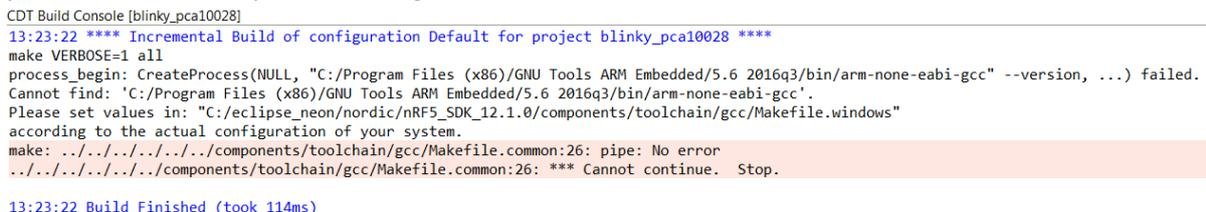
Figure 3: console output with SDK version 12 and later where the toolchain path is not set correctly. Should have been C:/Program Files (x86)/GNU Tools ARM/5.4 2016q3/bin/arm-none-eabi-gcc to correspond with this particular setup.
