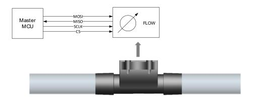
ESRF-ESF sensors have the option of a serial peripheral interface communication following the memory mapping as described in section 9. The sensor uses MODE 0 SPI with CPOL = 0 and CPHA = 0.
