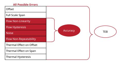
The figure below, illustrates the accuracy as well as the total error of the flow measurement of ESRF-ESF sensors.
