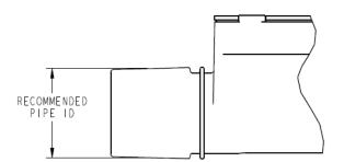
For optimal performance, the sensor requires at least 20x ID of laminarizing pipe length in the flow inlet and another 20x ID in the outlet. ESRF-ESF sensors are calibrated using 20mm ID pipe diameter. The diameter of the inlet and outlet flow pipes should be as close to the calibration diameter as possible. It is also possible to insert O-rings in the grooves and attach tubes with an inner diameter of 23 mm to the ESRF-ESF. The dimensions of the O-ring are illustrated bellow.
