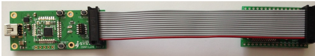
Fig. 4: Connecting IDAP-Link to the breakout board
