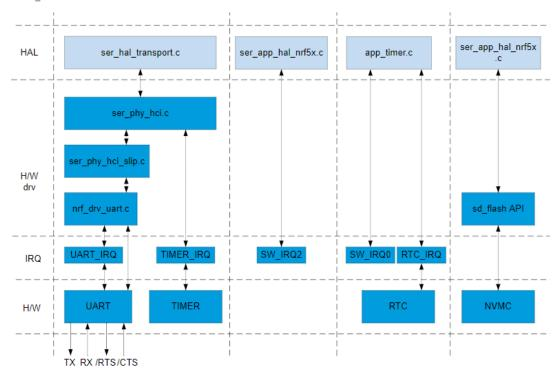
UART HCI means use of H5 protocol for UART communication, makes it more reliable, SLIP encoding.
