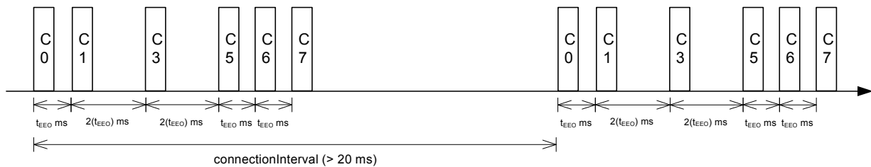
Figure 16 Multi-link scheduling - max connections, interval > min
