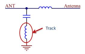
Resonant frequency between 2<sup>nd</sup> and 3<sup>rd</sup> harmonic
