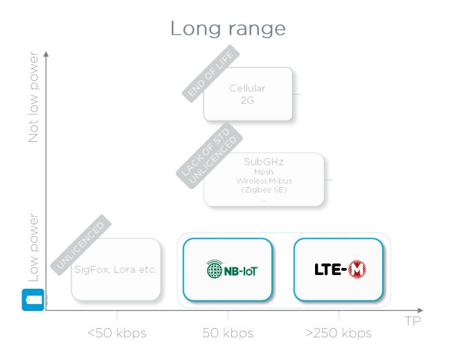
Cellular IoT (NB-IoT & LTE-M) is the ideal technology for utilities to connecting smart meters
