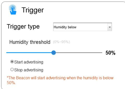
**Humidity threshold** – Alarm that triggers when the sensor humidity is *lower than* this value, and configuration range is 0%~95%.
