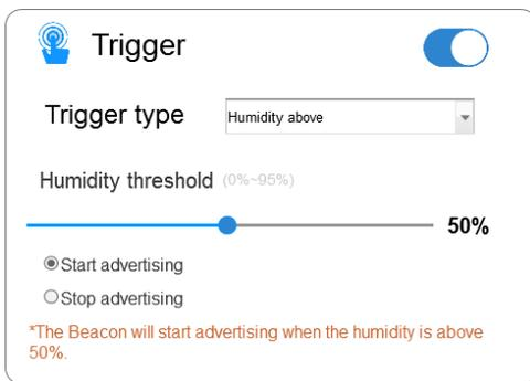
**Humidity threshold** – Alarm that triggers when the sensor humidity is *higher than* this value, and configuration range is 0%~95%.
