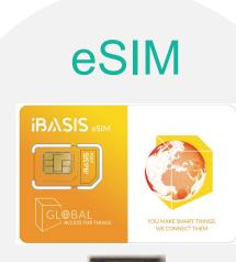
As the need arises, the device can be re-programmed remotely with a different set of operator credentials
