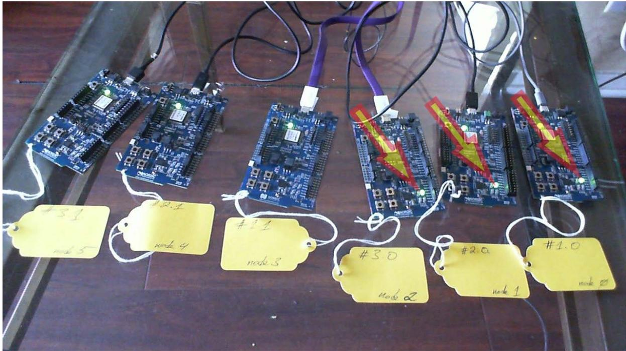
27. Now we turn off Application Key 0 Group LEDs and turn on Application Key 1 Group LEDs to show that node 3 is now back to being part of Application 0 Group:
