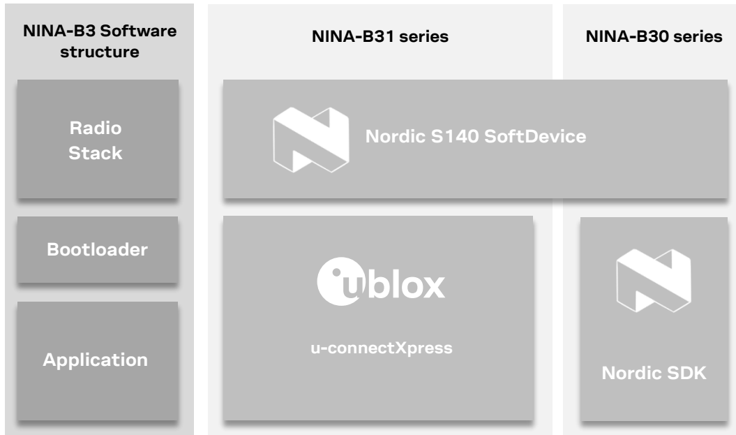
Figure 2: NINA-B3 software structure and available software options
