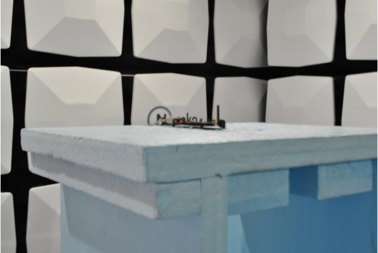
Radiated measurement set-up
