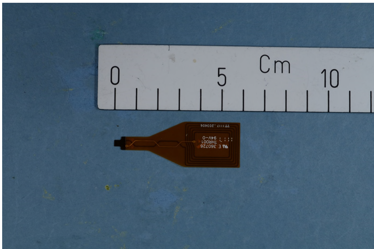
NFC antenna – front side
