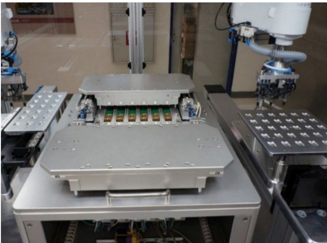
Figure 29: Automatic test equipment for module testing
